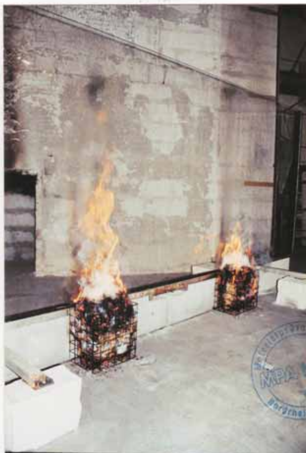
Fig. 2: Test wall during the fire tests
