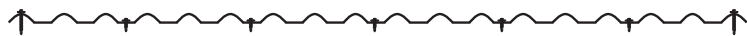
Positions for fastening roof or wall screws at internal purlin. Figure 10a
